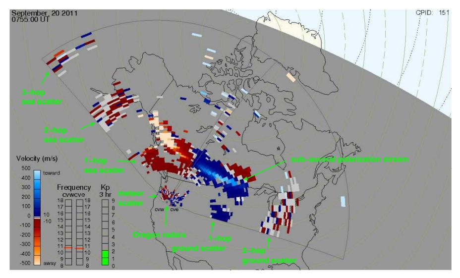
Backscatter from the Oregon radar pair (cvw and cve) showing a strong westward flow channel across Canada. This feature know as a sub-auroral polarization stream (SAPS) and is observed by the Oregon radars during geomagnetically disturbed periods. Backscatter at close ranges to the radars is likely from meteor trails or the E-region. 1-, 2- and 3-hop sea scatter is observed in the most westward looking beams of cvw and the first two hops in the most eastward looking beams of cve.
